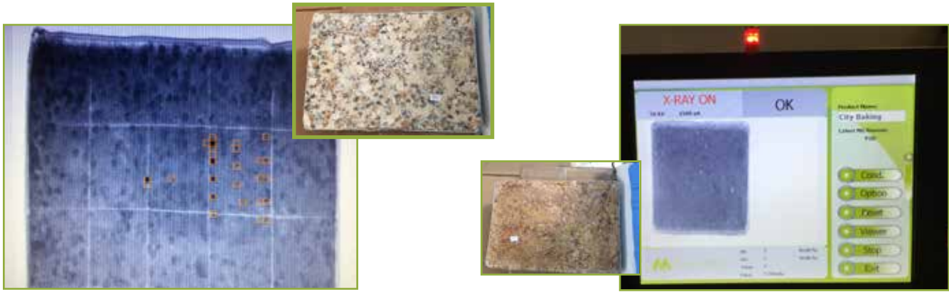
The system automatically stores reject images for HACCP traceability
