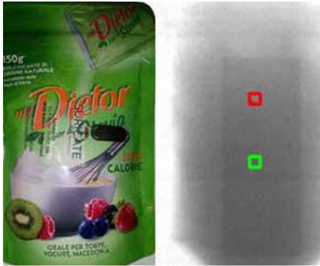
MEKI pinpoints contamination inside the liquid myDietor pouch. Stainless steel diameters are 0.6mm and 0.8mm.
