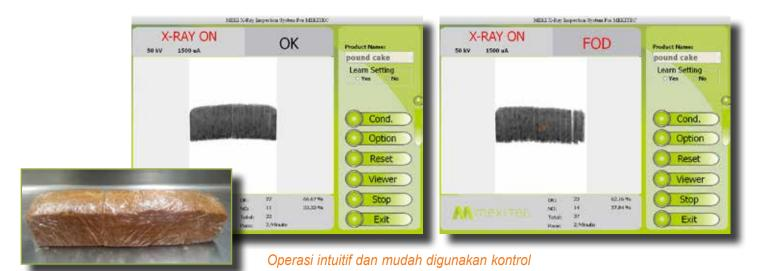
in the City Baking production line, where it can monitor baked goods that have already been baked, cut and prepared for consumption. Because X-ray technology enables in-foil scanning, no manual intervention is necessary to prepare goods for inspection. And, while City Baking production facilities are free of glass, ceramic, stone, and other dense materials, MIDMEKI is capable of detecting those contaminants on the off chance they're present. That's an insurance policy not offered
